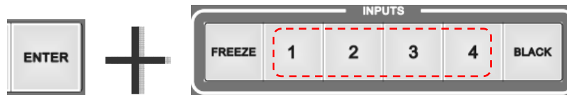
Figure 5-14 Shortcut Key Combination Transfer Operation Flowchart
